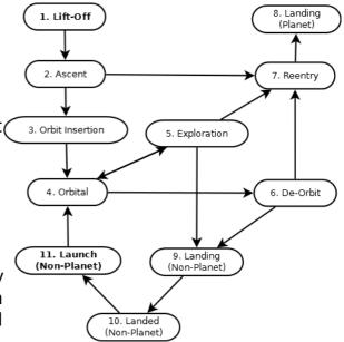
position in Space Dimension is calculated from the position of Launchpad. The next Phase is 4. Active Component: Second Booster Stage
